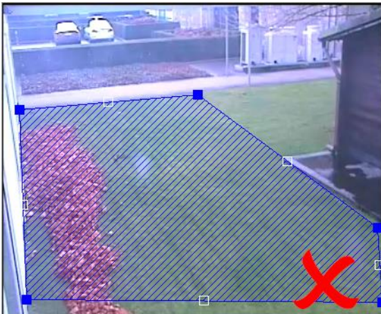
Detection zone does not reach edge of image. Warning! IntrusionTrace may not detect intruders in the foreground because their path can pass below the detection zone.
