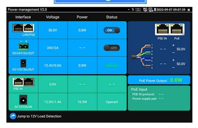
Measurement POE switch or PSE power supply voltage and cable connection status. Measurement POE switch or PSE power supply voltage and cable connection status. View real-time data such as voltage and power of POE, DC12, DC24V output/PSE, and DC12V input.
