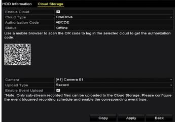
Figure 12-20 Upload to Cloud Storage Interface
