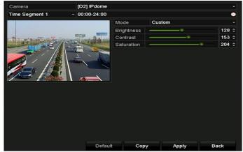
Figure 13-6 Image Settings Interface (IP Camera)
