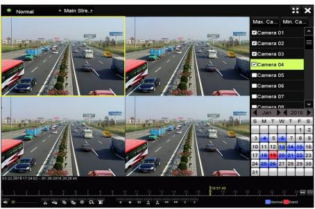
Figure 6-24 4-ch Synchronous Playback Interface
