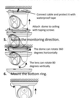
Push bottom ring back up and turn it clockwise to lock into position
