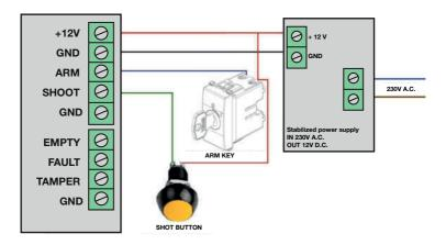
In the diagram above Ur Fog is powered by an external power supply.
