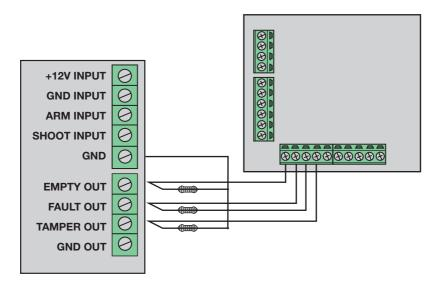
In this diagram, putting the resistance value required by the alarm control panel used in the terminal UR Fog, with not used outputs the central will see the correct resistance, while following the activation of an output, you will have a pull-down causing the alarm of the corresponding zone.
