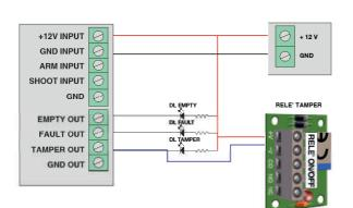
In case of an empty cylinder, the DL EMPTY led will switch on.
