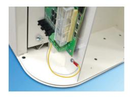
While connecting the machine to the mains power, it is raccomended to never disconnect existing ground cable. The fact of disconnecting or modifing existing cables voids the warranty and can cause troubles or accidents related to the temperature control.
